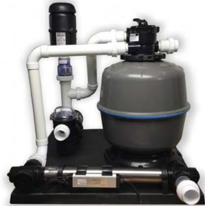
Step 3: Attach the ZapTek UV to the filter outlet as shown. Attach pipe to pump and inlet of filter. Hand tighten only the unions. Make sure the gaskets are in the unions at the connections.
