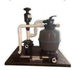
Step 2: Set the filter, pump and UV on the pad as shown. Place media Agitator on Check valve. Do not glue Agitator to pipe. Use a set screw through the pipe and agitator throat if needed to hold it. Connect like number to like number by tightening the unions together by hand.
