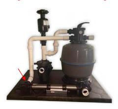
Step 3: Attach the ZapTek UV to the filter outlet as shown. Attach pipe to pump and inlet of filter. Hand tighten only the unions. Make sure the gaskets are in the unions at the connections.
