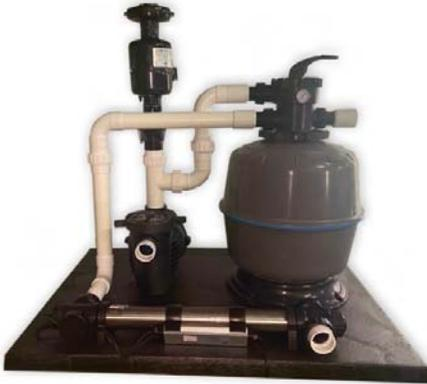
Step 2 : Set the filter, pump and UV on the pad as shown. Place media Agitator on Check valve. Do not glue Agitator to pipe. Use a set screw through the pipe and agitator throat if needed to hold it. Connect like number to like number by tightening the unions together by hand.
