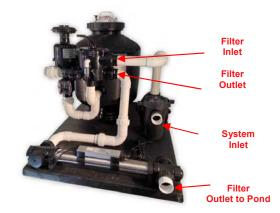
Step 3: Attach the ZapTek2 UV to the filter outlet as shown. Attach pipe to pump and inlet of filter. Hand tighten only the unions. Make sure the gaskets are in the unions at the connections.
