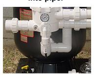
After double checking all connections to make sure they are tight you are ready to prime and start the system. We recommend that a "SWING" check valve be installed below surface grade of pond on intake into the system. This will make the priming of the system a snap. To Prime system, fill AquaSieve (if so equipped) with water and pump with water. Close the units and start pump.
